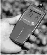
A more accurate measurement can be achieved by holding on to a ground point like a ground wire, grounded metal pole etc. with your other hand while taking a measurement.
