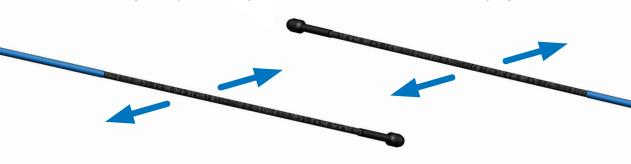
**4.** For model AA-SGS/25, the 2.5m version, the fibreglass rods come in two pieces that have to be connected using the nuts and bolts provided before you can use the gate.
