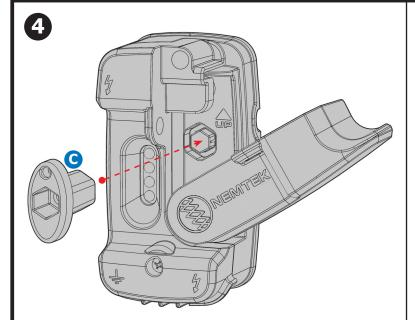
As a safety feature, the lever arm can be 'locked' open (OFF position) using the terminal nut tool (C) to prevent accidental closing of the lever arm (ON position) when working on the fence
