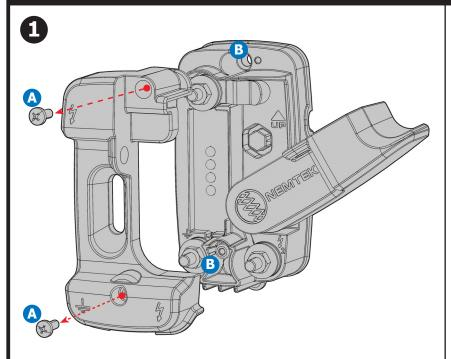
Remove the two screws (A) at the top and bottom of the switch and take off the switch cover to expose the mounting holes (B)
