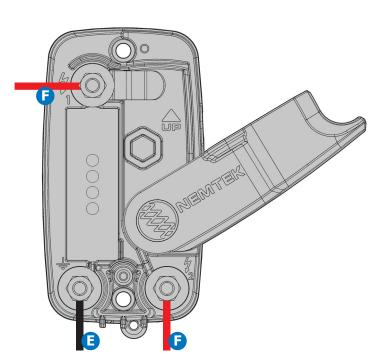
For the AA-COS/LED model, one earth wire (E) and two live wires (F) need to be connected
