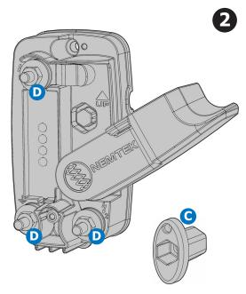
Mount the unit onto your preferred surface and use the terminal nut tool supplied (C) to loosen the nuts on the terminals (D)
